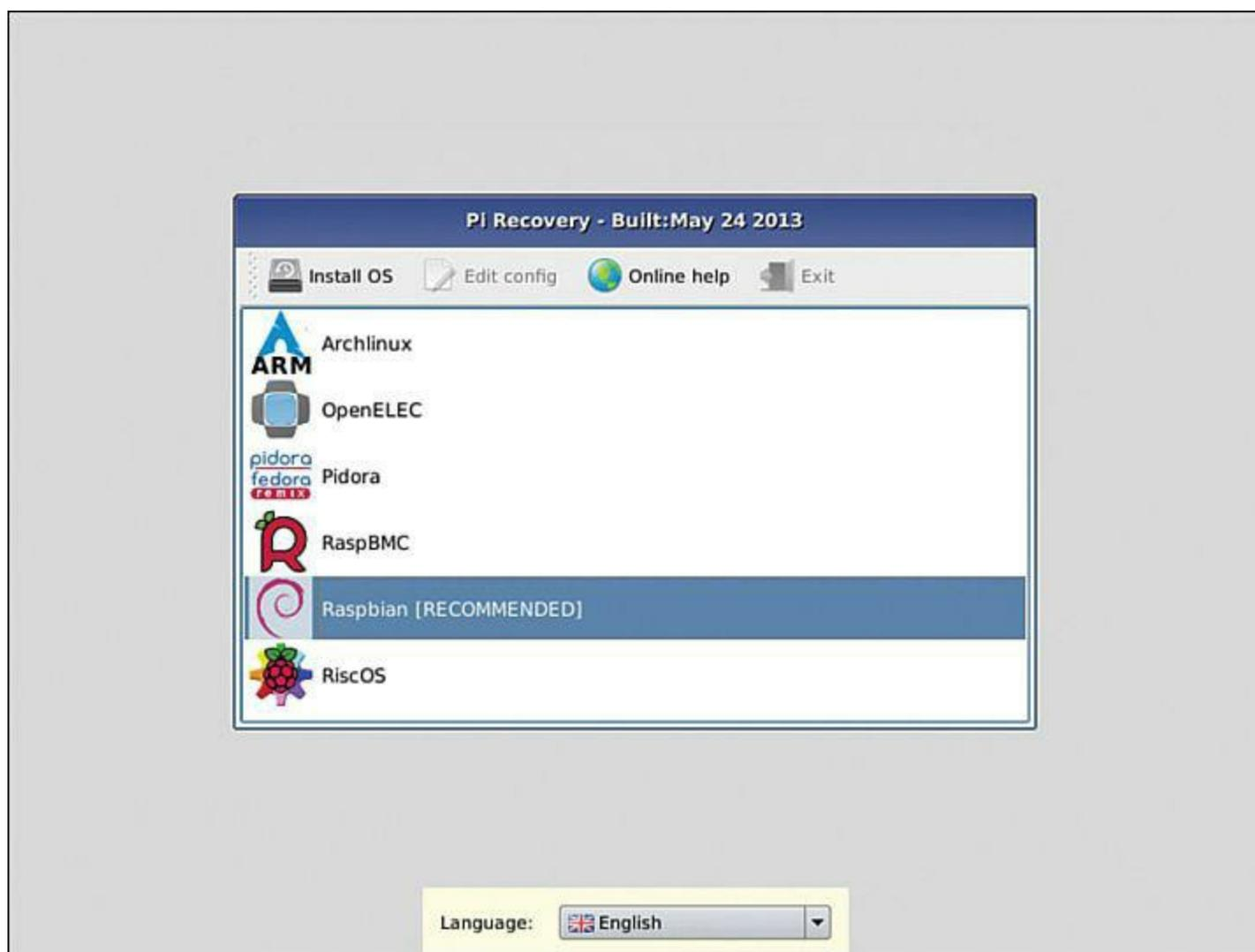
**FIGURE 4.11** The NOOBS utility makes it much easier to load an OS on your Raspberry Pi.
